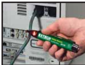
Locate power cord breaks
