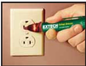
Line outlet testing
