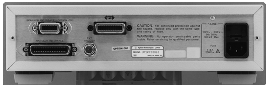
Rear panel of the Agilent 4268A 120 Hz/1 kHz capacitance meter (with Option 4268A-001)
