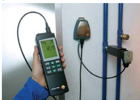
Precision meter for any parameters: Testing a transmitter with 0/4 ... 20 mA interface
