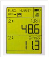
Automatic calculation of different humidity parameters in the instrument
