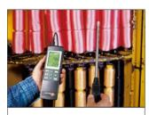
Measuring humidity at up to +180°C in drying systems
