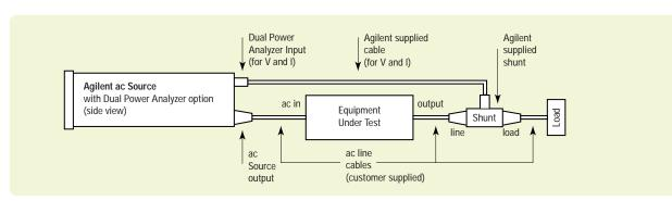
Test configuration of efficiency measurement using an Agilent ac source with the 020 Dual Power Analyzer Option.
