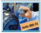
testo 905-T2 The sprung, wide thermocouple measuring head, type K, guarantees a very quick reaction time and a high accuracy level by placing the probe flat on the uneven surface.
