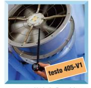
testo 405-V1 is the first mini anemometer in this price range which can measure air velocity and volume flow
