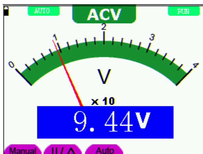
Figure 26: AC Voltage Measurement
