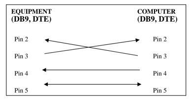
Figure 2 Wiring configuration for DB9 to DB9
