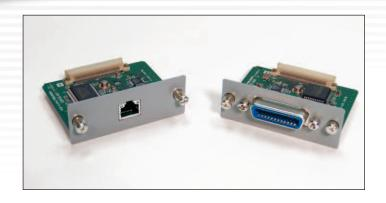
back to the controlling PC. Both ScopeExplorer and ActiveDSO are available for free download from LeCroy's Web site. The WJ-LAN and WJ-GPIB interfaces are automatically recognized by, and are compatible with, all WaveJet oscilloscopes running firmware version 3.06 or greater.
