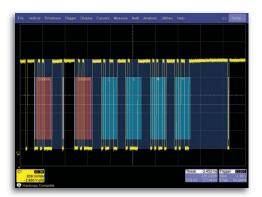
specific events on your embedded controller. Trigger on DATA in specific locations of long I<sup>2</sup>C EEPROM reads, or trigger on sensor values outside of a certain range. Intuitive, color-coded decode overlay helps you understand your serial data signals quickly. Search for data patterns, or view the protocol data in a table. Export table data to Excel.
