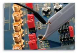
A variety of standard and available probe tip and grounding accessories are offered to meet any requirement. What's more, ZS Series probes are available for a very affordable price. The ZS1500, 1.5 GHz probe gives full 1 GHz system bandwidth at the probe tip when used with the WaveRunner 104MXi.
