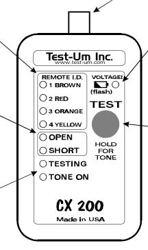
**VOLTAGE! LED** If voltage is detected this LED will light. (DISCONNECT IMEDIATELY!) LED also indicates low battery when flashing. Replace battery to ensure proper operation.
