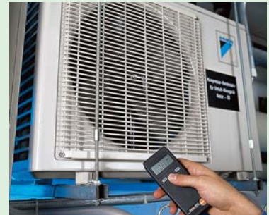
Measurements at inaccessible points using testo 465
