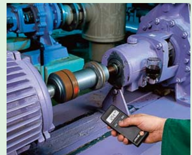
rpm measurement on shafts, rollers etc. using testo 465
