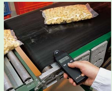
Speed/length measurement using testo 470
