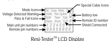
Instructions for Use Resi-Tester<sup>TM</sup> powers off automatically 9 minutes after the last button press in cable testing modes and after 2.4 hours in tone mode. Be sure to install a battery if using for the first time, see battery installation section.
